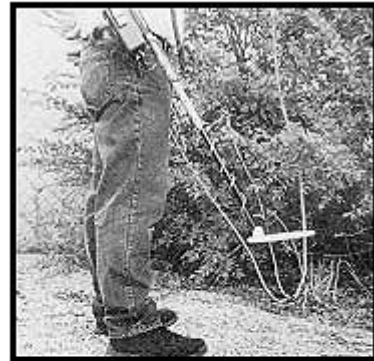
Lift your detector straight off of the ground about 6 to 8 inches. Keep the coil parallel to the ground.
