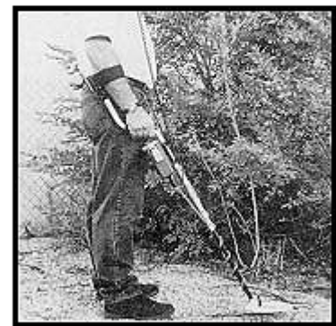
Once you have got a steady threshold, quickly lower the coil straight down to approximately 1 inch off of the ground.
