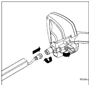
Figure 2.6 Attaching coil cable to control box
