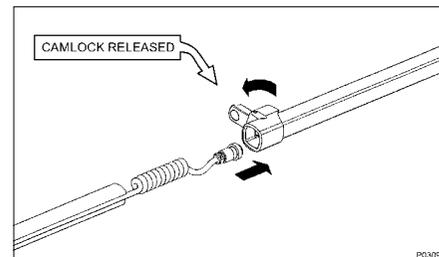
Figure 2.4 Feeding coil cable into upper shaft
