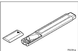
Figure 3.2 Replacing alkaline batteries
