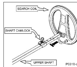
Figure 2.5 Sliding lower shaft into upper shaft
