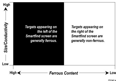
The Explorer rates detected objects according to their conductivity (like most traditional detectors). What makes two-dimensional discrimination unique is a rating of the same object's ferrous content. Smartfind graphically represents both of these target properties on the same display.
