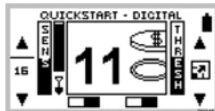
Figure 5.7 Quickstart's Digital display
