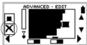
Figure 6.11 Rejecting framed target area
