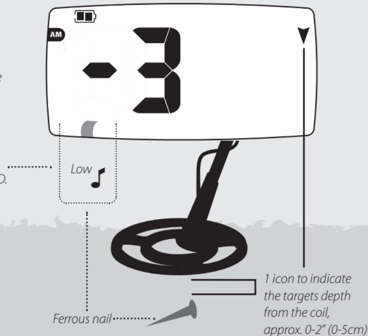
Metal detectors work due to the fact that metal is conductive. Metal detectors create an electromagnetic field, which penetrates the ground.
