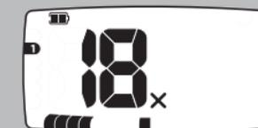
Custom patterns are saved when the X-Terra is switched off. To erase custom patterns and return to preset patterns:
